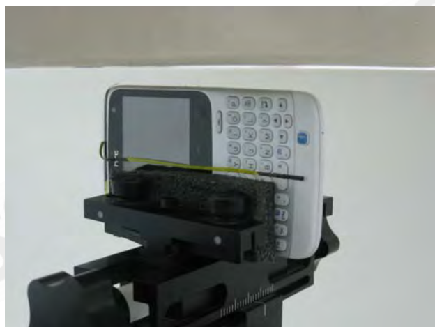
Fig.11 Body worn- EUT Right to flat phantom and distance between flat phantom and mobile phone is 1 cm.
