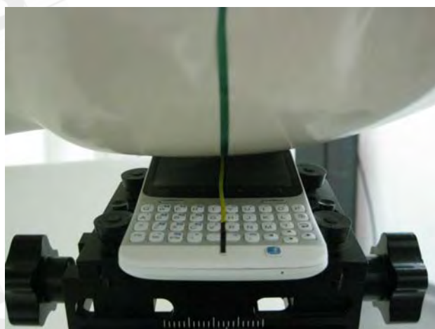
Fig.6 Left Head Section / Ear-Tilt Position(15°)
