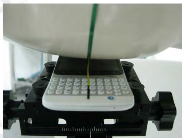
Fig.4 Right Head Section / Ear-Tilt Position(15°)
