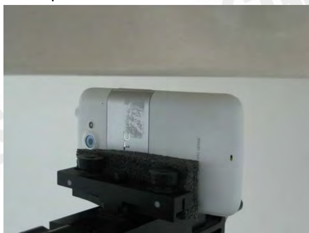
Fig.12 Body worn- EUT Left to flat phantom and distance between flat phantom and mobile phone is 1 cm.
