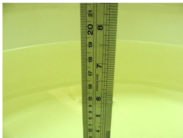
Fig 6.2 Photo of Liquid Height for Body SAR
