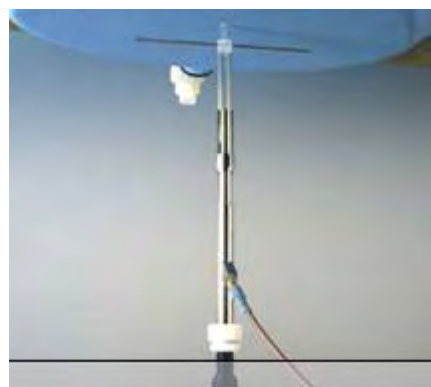
Photograph of the dipole Antenna
