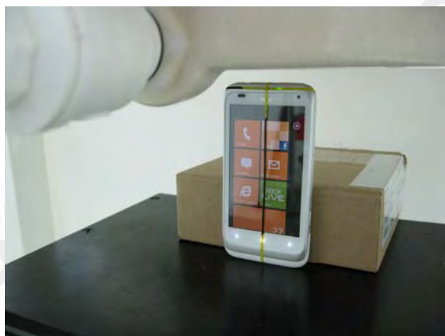
Fig.9 Hotspot mode- EUT Top to flat phantom and distance between flat phantom and mobile phone is 1 cm.
