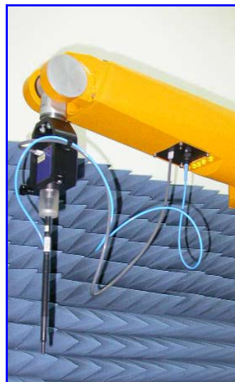
Figure 4. Probe setup on robot
