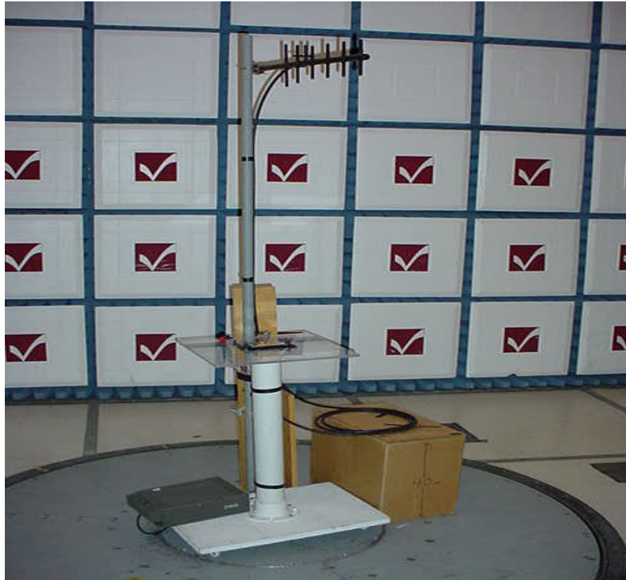
Setup for the Radiated Emissions Test, view with yagi transmit antenna (Case #1)
