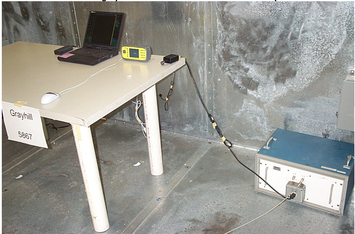
Photograph of Conducted Emissions Test Setup
