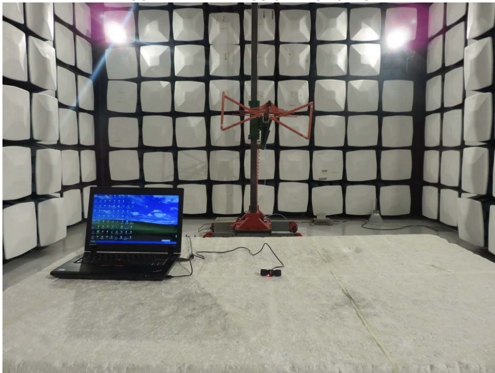
FCC RADIATED EMISSION TEST SETUP
