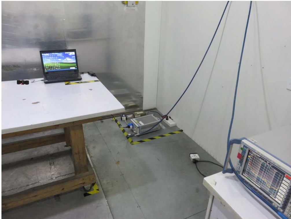
FCC RADIATED EMISSION TEST SETUP
