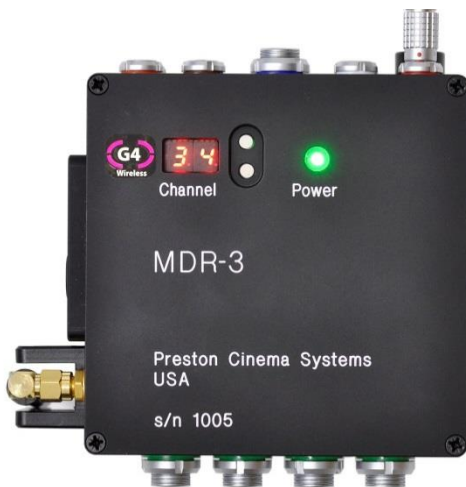
MDR3: Channel Display & Switches – Top
