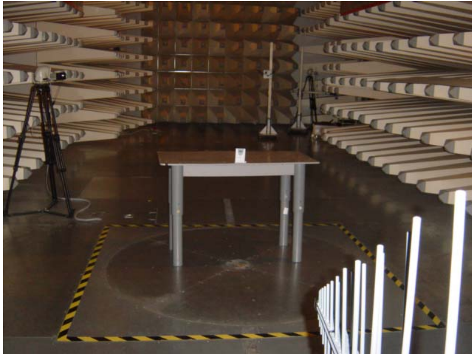
Set-up for Radiation Emission (Transmitter)
