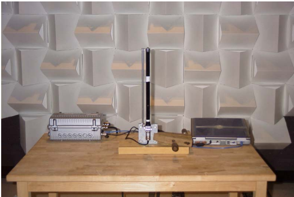
Radiated Emission Test Setup – KA-00 Antenna
