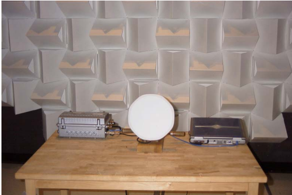
Radiated Emission Test Setup – WNA-202F Antenna
