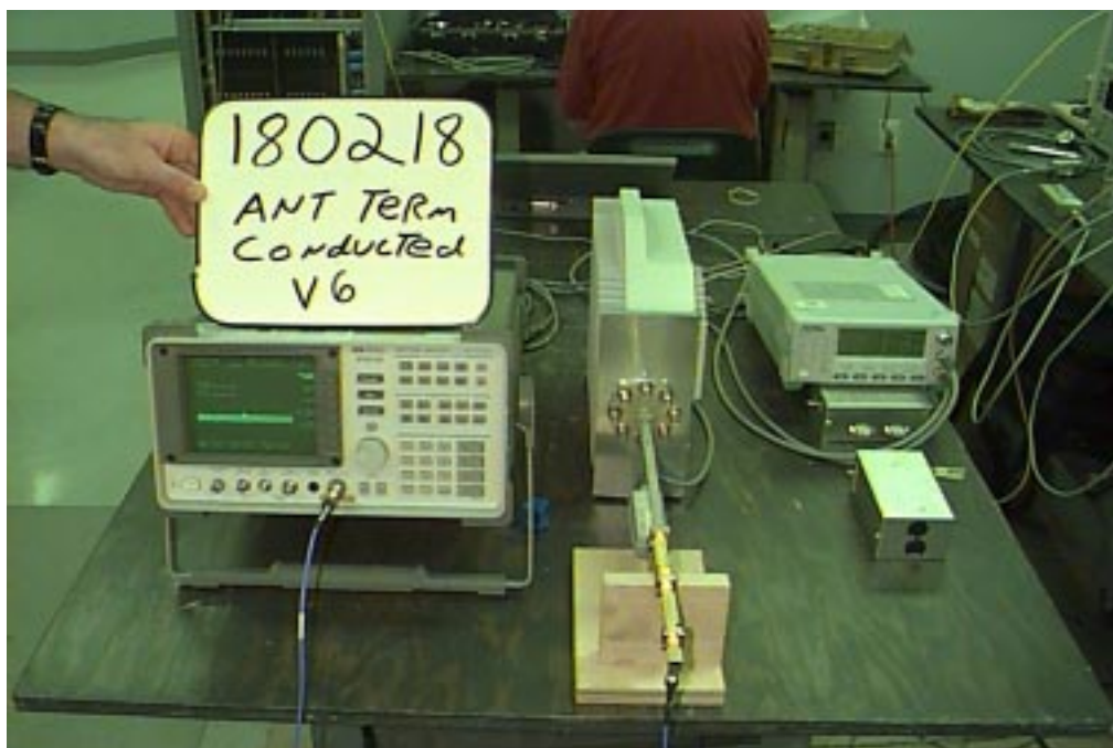
FIGURE D-3. ANTENNA TEMINAL CONDUCTED EMISSIONS TEST SETUP (Conducted)
