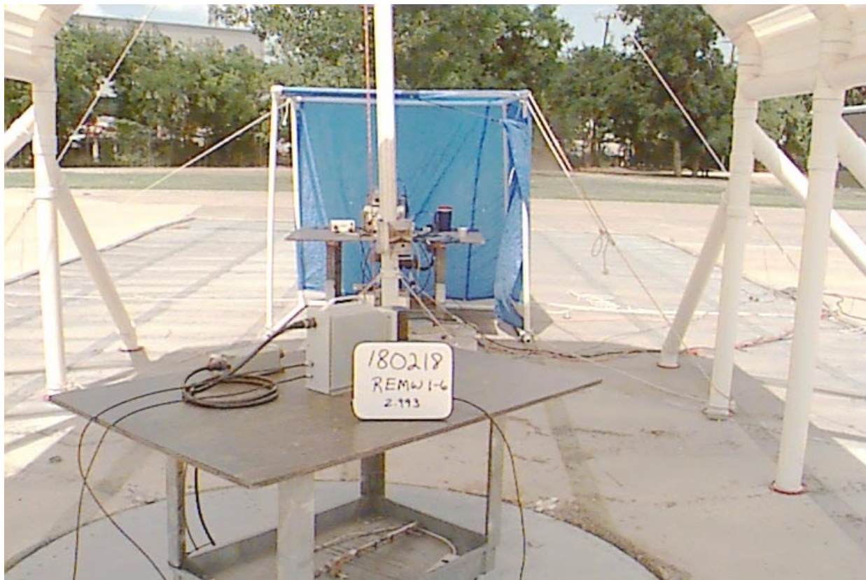
Figure 7-4 Test Setup for Spurious Radiated Emission Measurements
