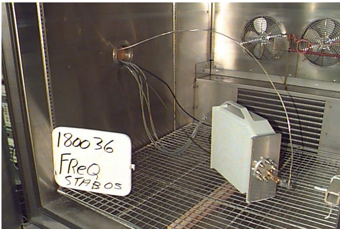
Figure 7-5 Test Setup for Temperature Stability Measurements
