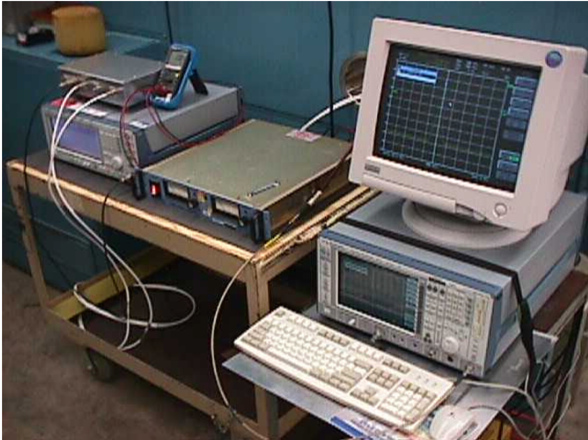
Figure 7-6 Setup for frequency stability measurements - equipment
