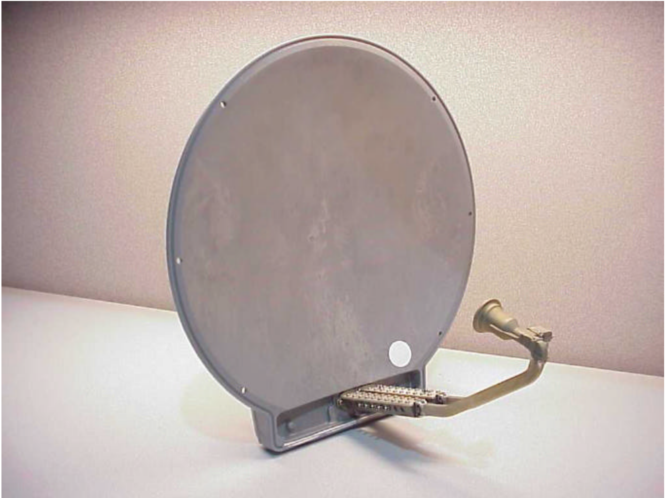
Figure 9-4 CPE Roof Unit With Radome Removed
