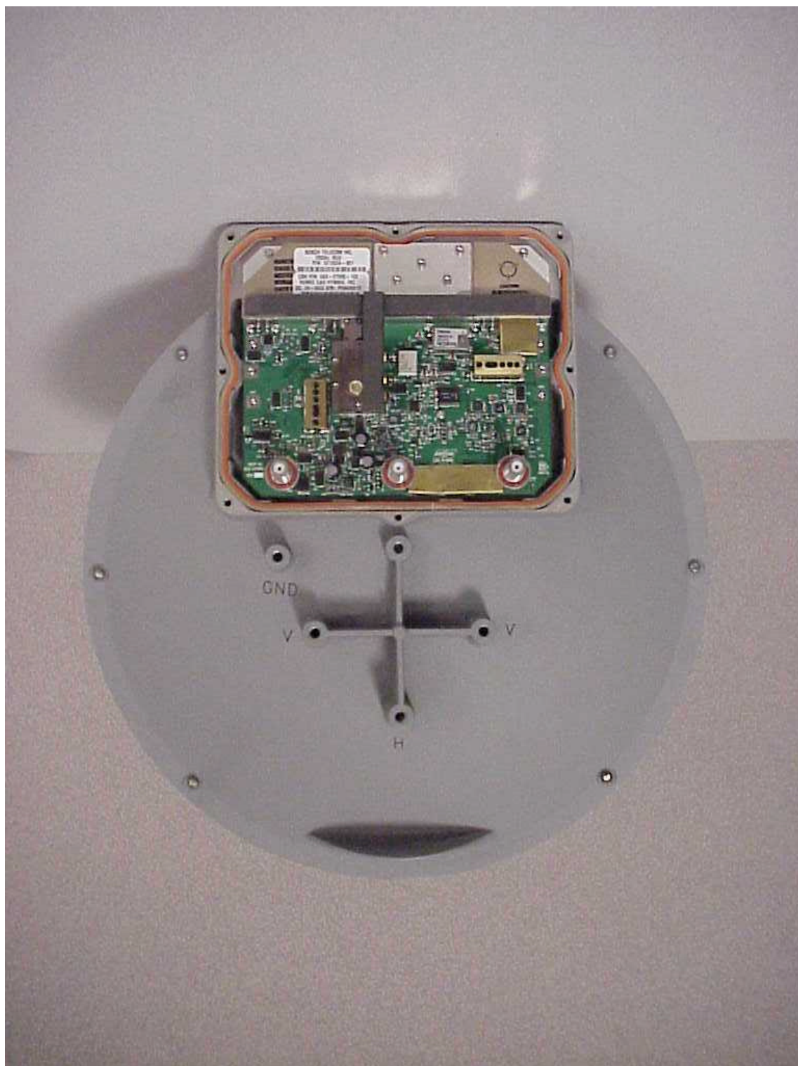
Figure 9-2 CPE Roof Unit with Electronics Board - Cover Removed
