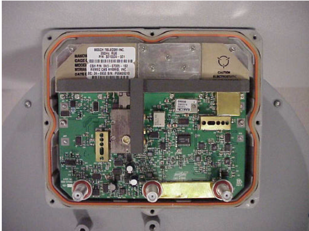
Figure 9-3 CPE Roof Unit with Electronics Board - Cover Removed (Close up view)
