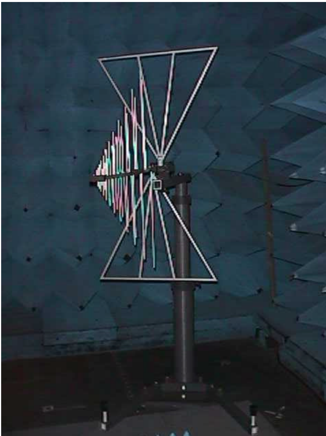
Figure D – 2 Setup of BiConiLog Antenna for Measurement of Radiated Spurious Emissions from the SpectraPoint CPE Roof Unit Transceiver
