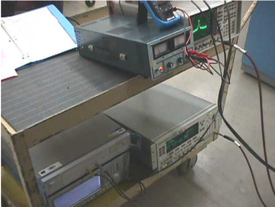
Figure 7-5 Setup for frequency stability measurements - equipment
