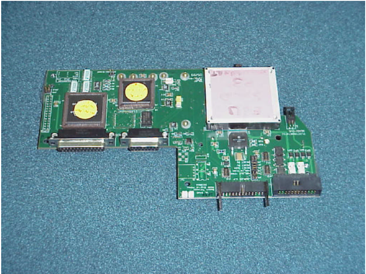
Figure 9-4 Node Transmitter Digital Board – Top side
