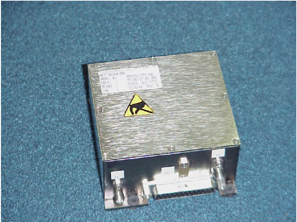
Figure 9-3 Node Transmitter Local Oscillator
