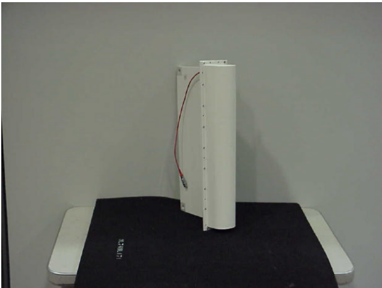
Figure 9-8 Node Transmitter Antenna assembly
