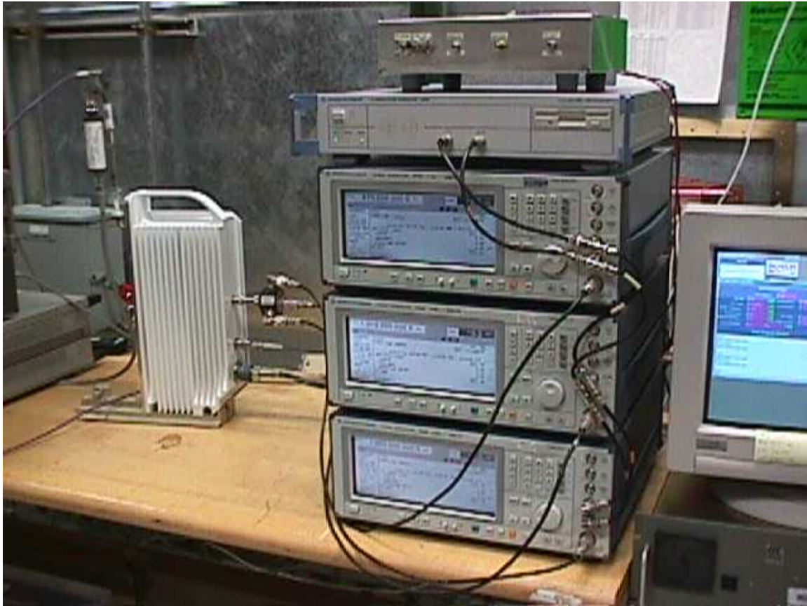
Figure A – 8 Test Setup for RF Power Spectral Density Measurements on the SpectraPoint High Gain Node Transmitter (view 2).
