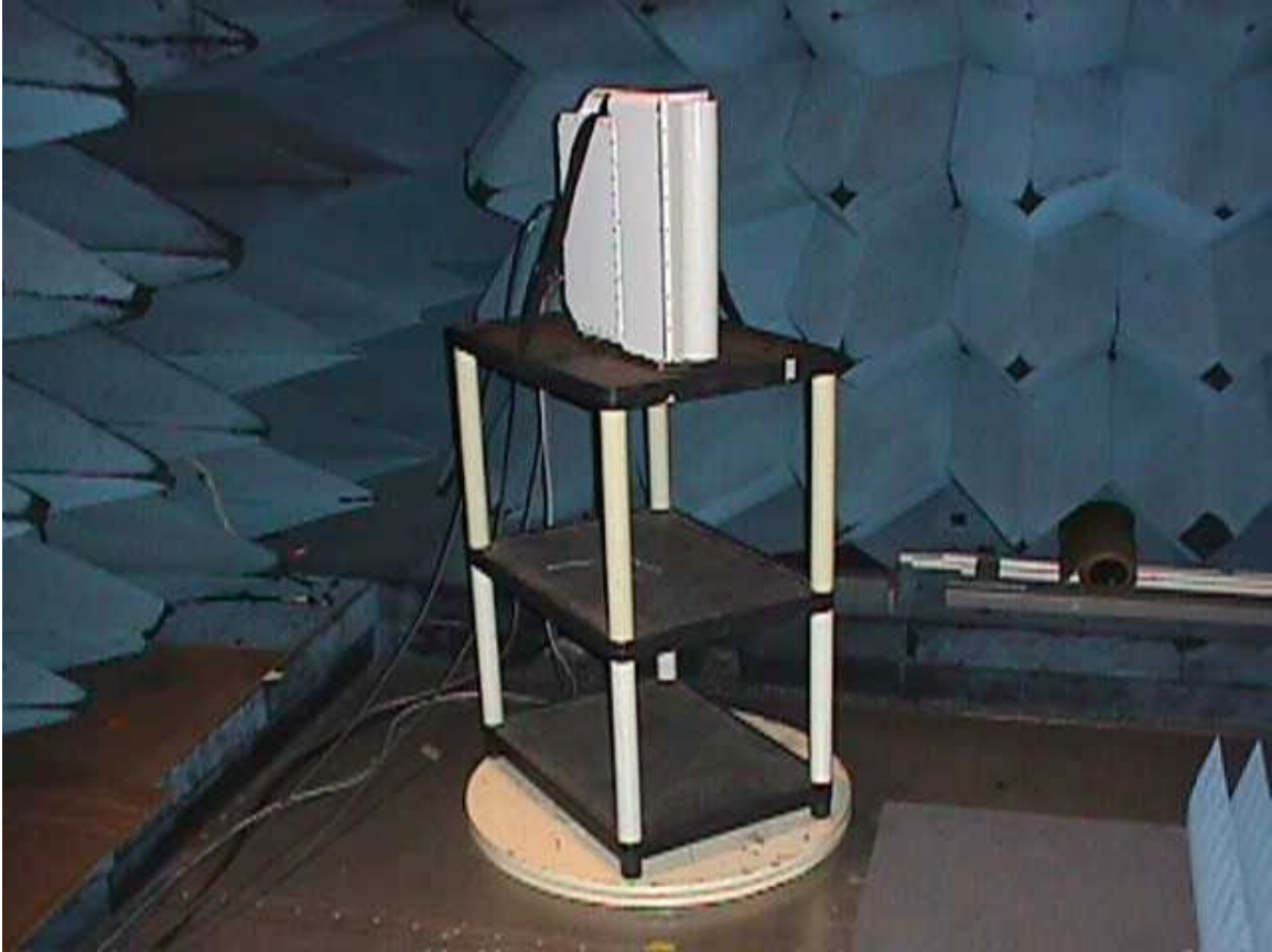
Figure D – 1 SpectraPoint High Gain Node Transmitter Setup for Radiated Spurious Emissions Testing
