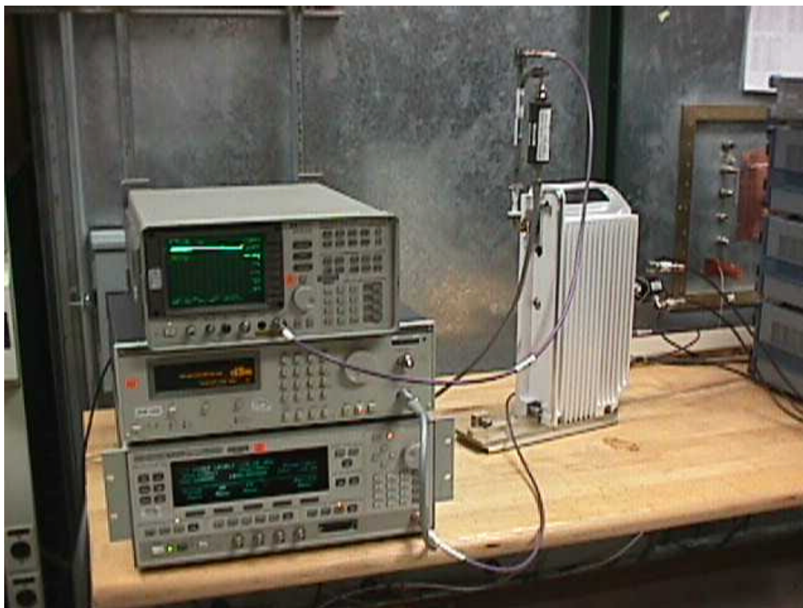
Figure C – 7 Test Setup for Antenna Conducted Measurements on the SpectraPoint High Gain Node Transmitter (view 1).
