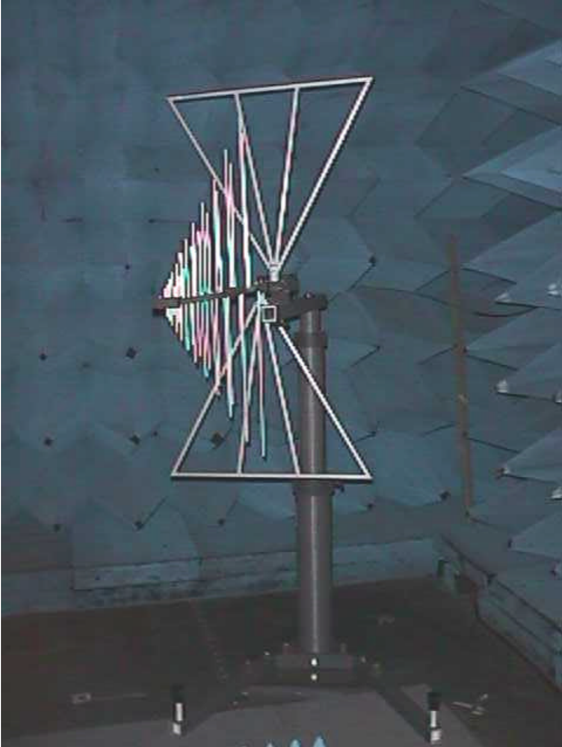
Figure D – 2 Setup of BiConiLog Antenna for Measurement of Radiated Spurious Emissions from the SpectraPoint High Gain Node Transmitter.
