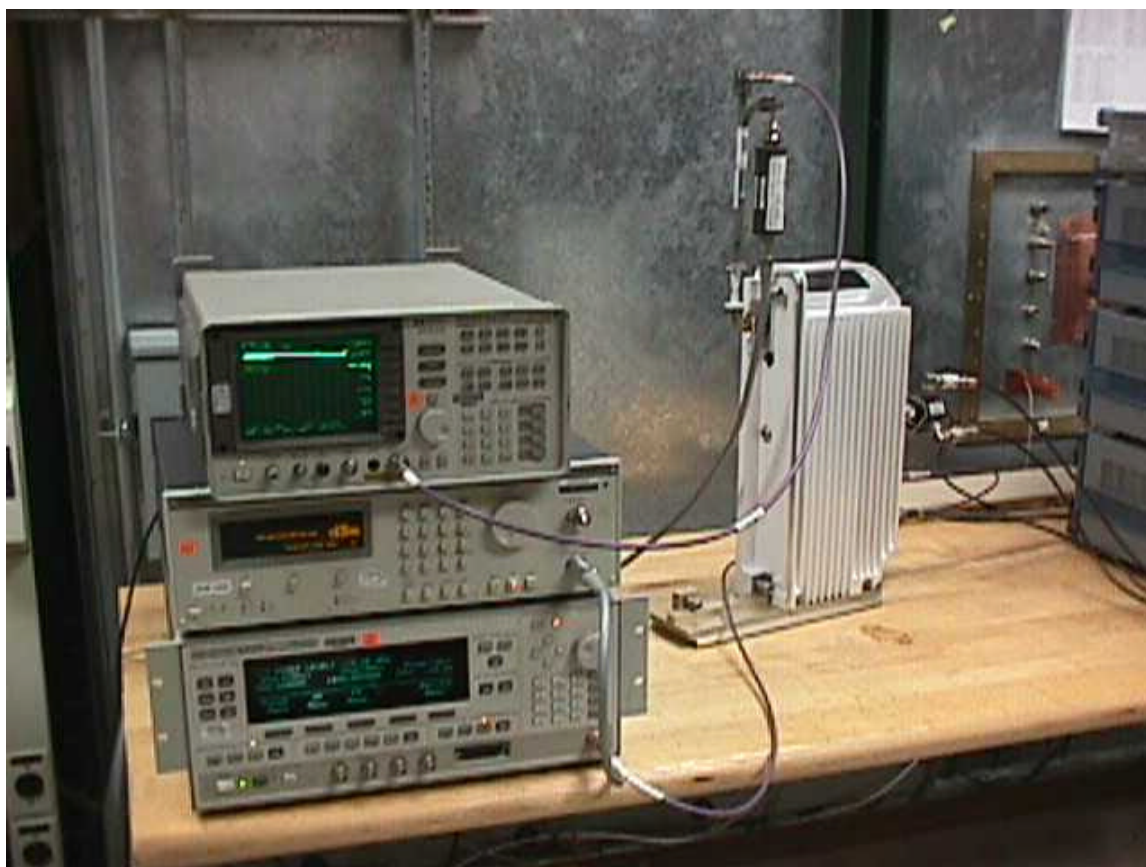
Figure A – 7 Test Setup for RF Power Spectral Density Measurements on the SpectraPoint High Gain Node Transmitter (view 1).
