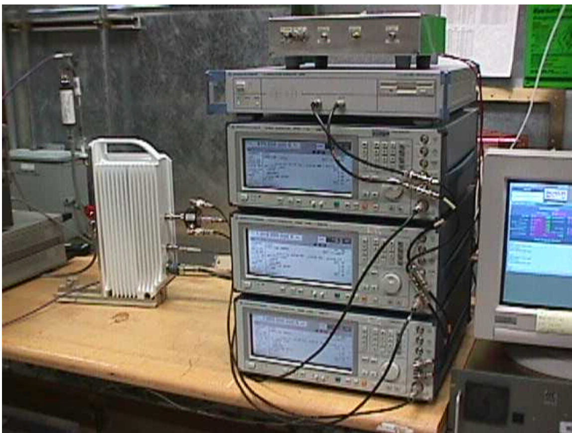
Figure B – 8 Test Setup for Occupied Bandwidth Measurements on the SpectraPoint High Gain Node Transmitter (view 2).
