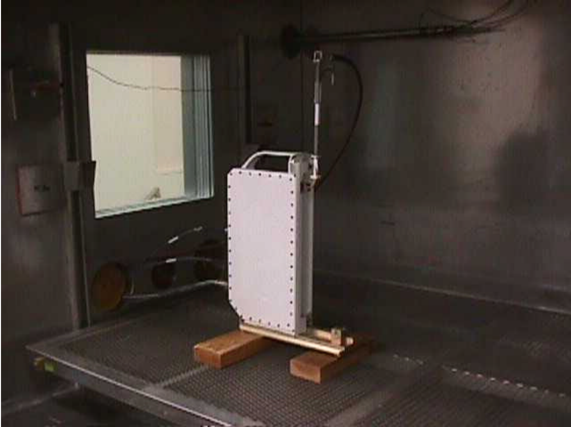
Figure E – 2 SpectraPoint High Gain Node Transmitter Setup for Frequency Stability Testing in the Temperature Chamber
