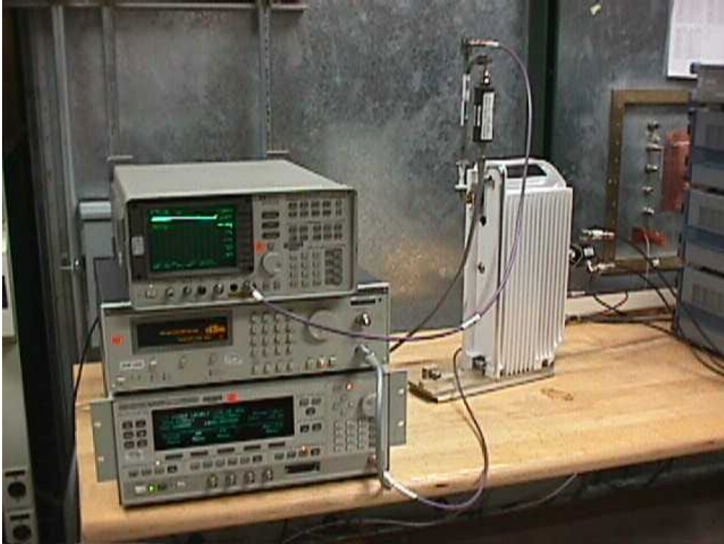
Figure 7-1 Test Setup for RF Power Spectral Density, Occupied Bandwidth, and Conducted Spurious Emissions Measurements on the SpectraPoint High Gain Node Transmitter (view 1)
