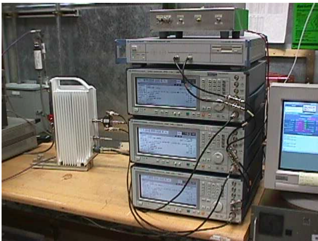
Figure 7-2 Test Setup for RF Power Spectral Density, Occupied Bandwidth, and Conducted Spurious Emissions Measurements on the SpectraPoint High Gain Node Transmitter (view 2)
