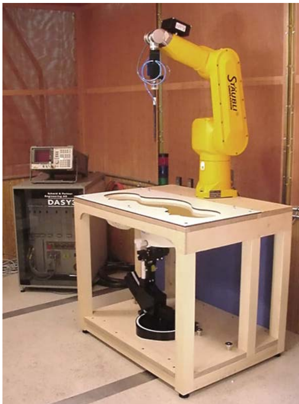
DASY3 SAR Measurement System with SAM phantom
