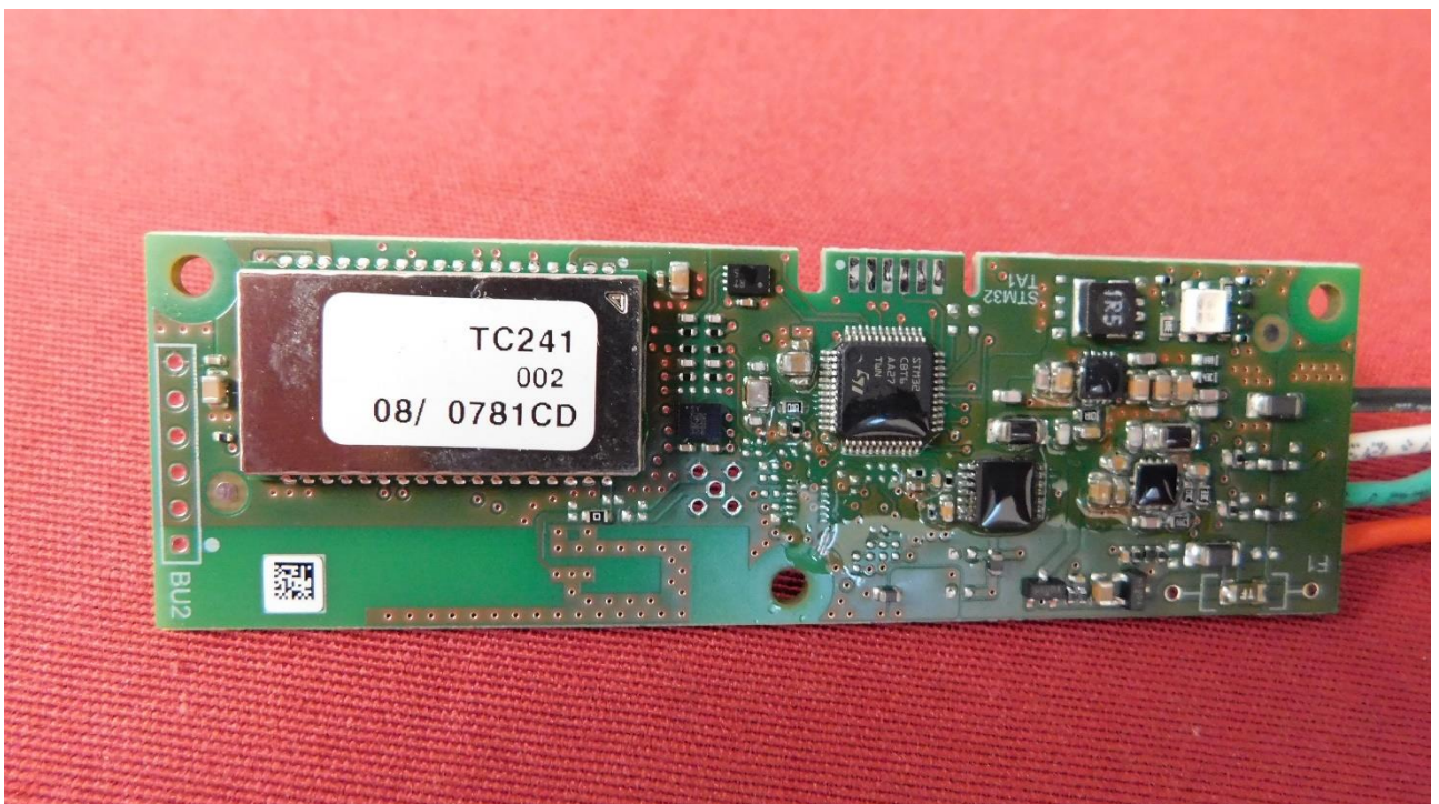
Picture 6: PCB of final product (not tested) – top side – with shielding
