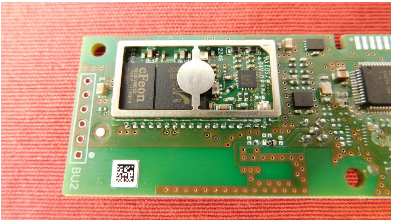
Picture 4: RF part of the EUT without shielding
