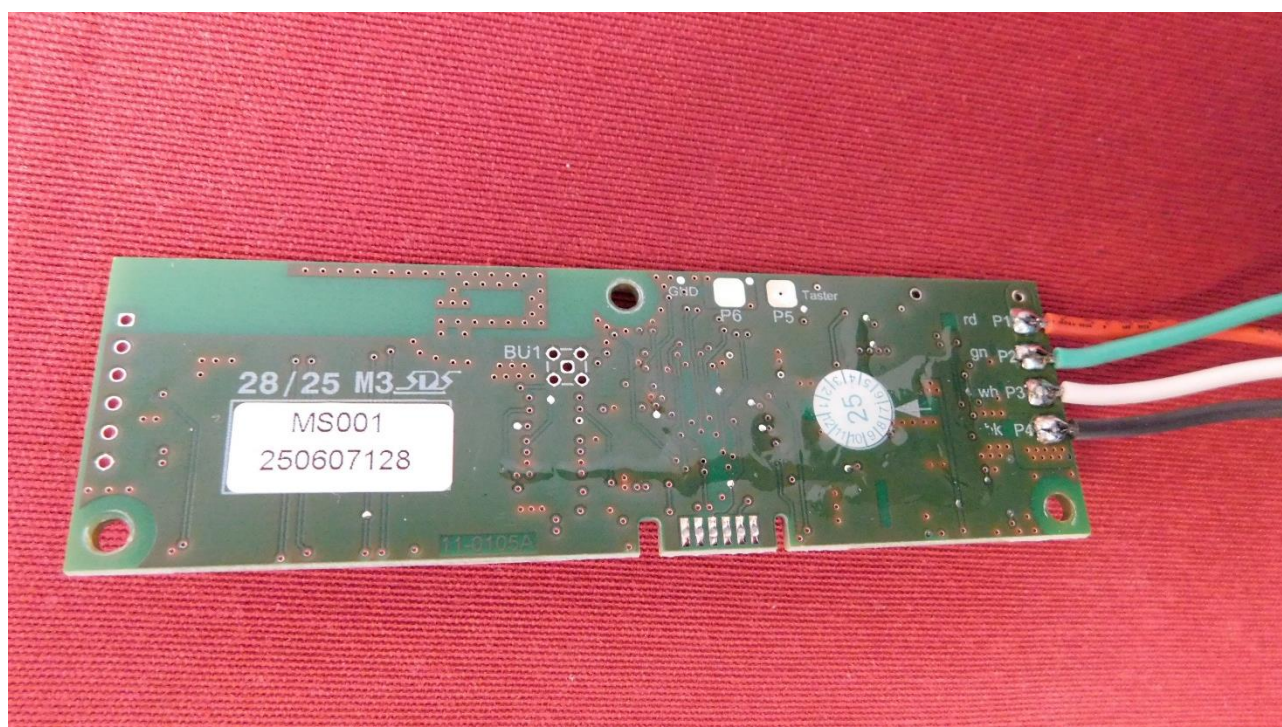
Picture 8: PCB of final product (not tested) – bottom side – without temporary antenna port
