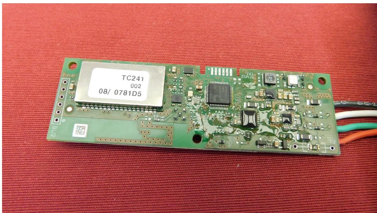
Picture 2: PCB of the EUT - top side, with shielding
