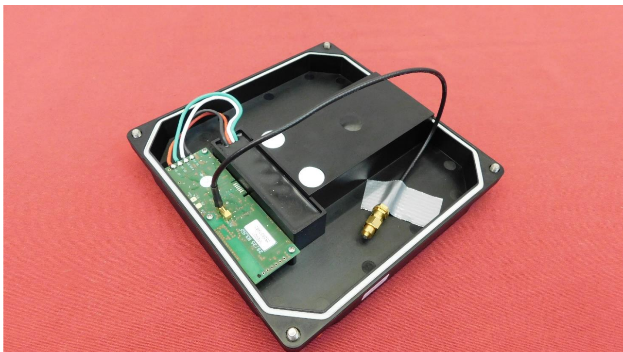
Picture 1: PCB of EUT - opened housing – with temporary antenna port
