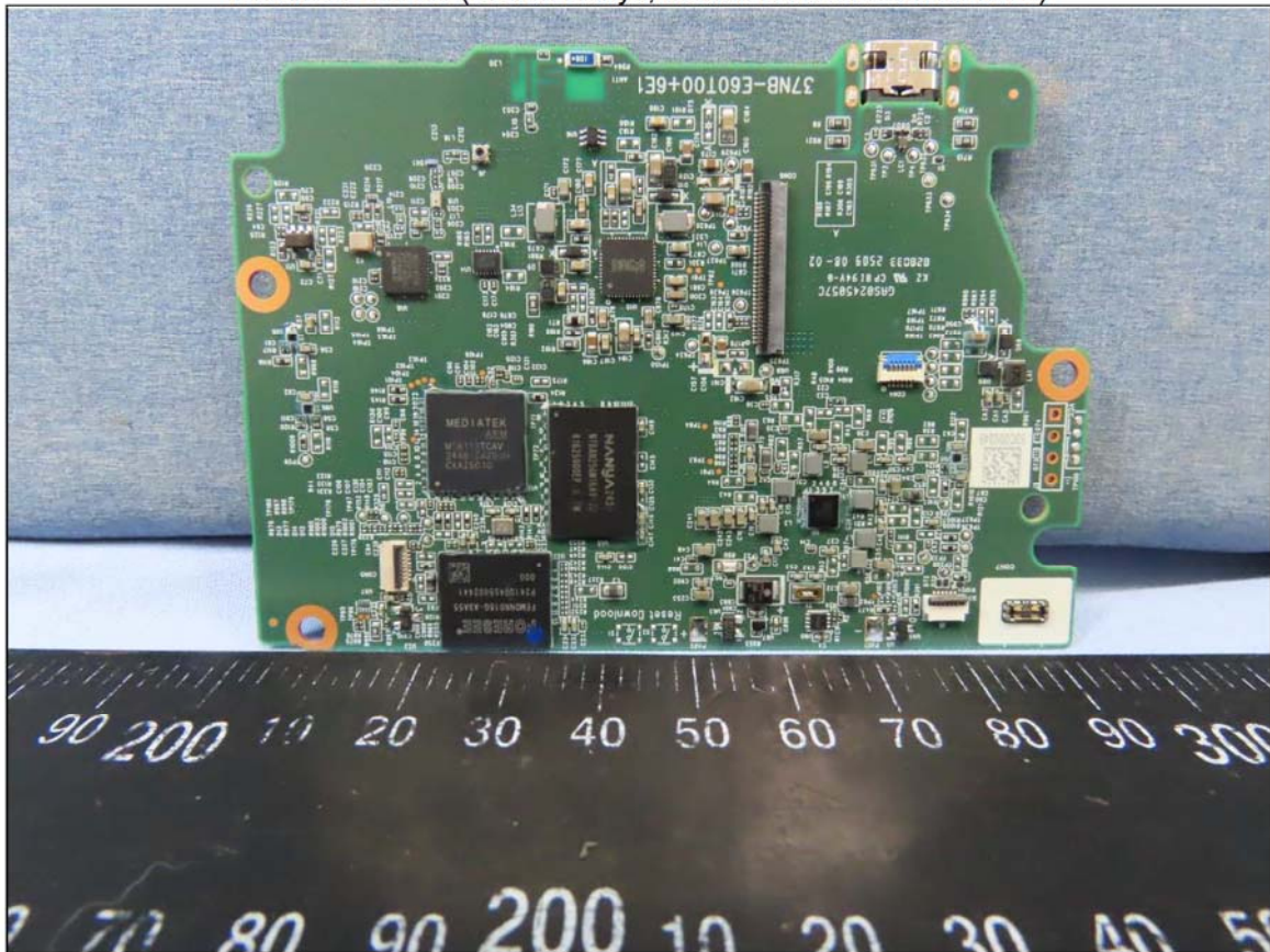
PCB with eMMC (Brand: FORESEE, Model: FEMDNN016G-A3A55) and DRAM LP-DDR4 (Brand: Nanya, Model: NT6AN256M16AV-J2)
