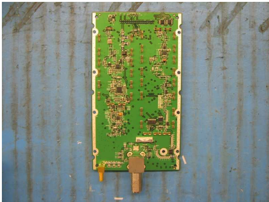
PCB Assembly Top View Ant Port without shielding - MRAU
