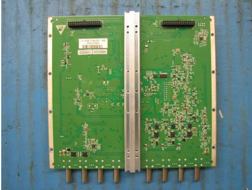
PCB IF Assembly Top View - MRAU
