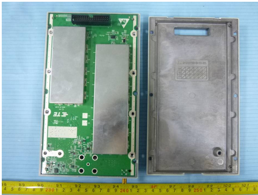
EUT – 800 MHz Band Cover off View
