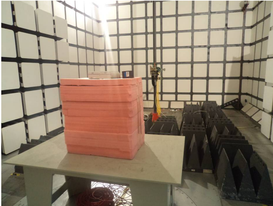
Transmitting Radiated Emissions – Front View (Above 1 GHz)
