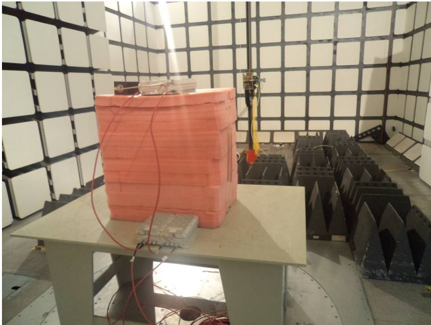
Transmitting Radiated Emissions – Rear View (Above 1 GHz)
