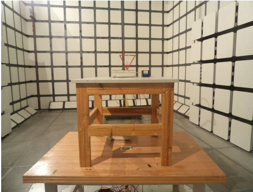
Transmitting Radiated Emissions – Front View (Below 1 GHz)
