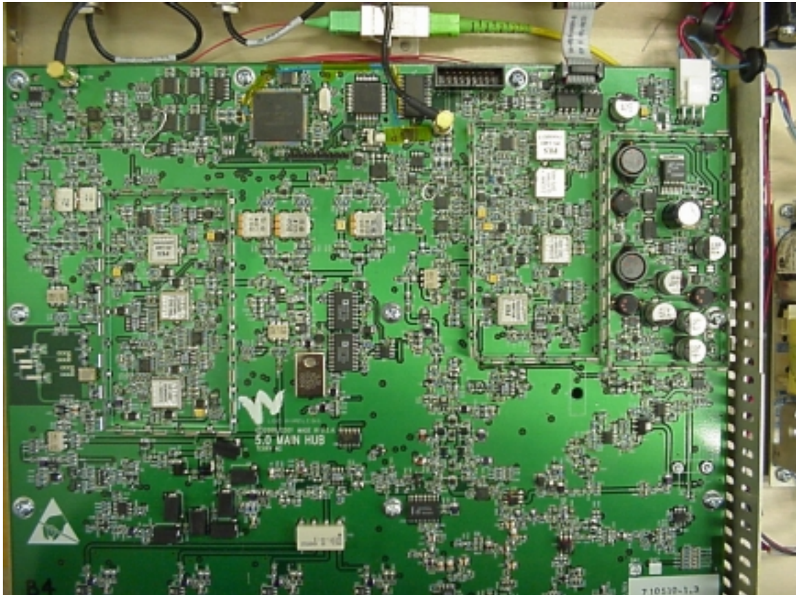
Inside of main hub (without shields)
