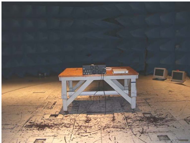
Photograph 5. Radiated Emission Limits Test Setup, 30 MHz to 1 GHz, Back View
