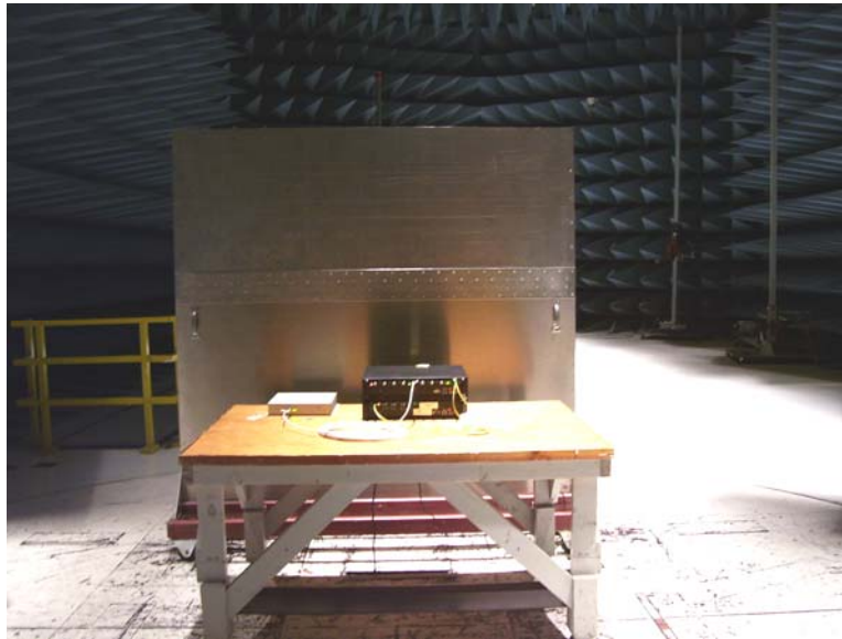
Photograph 2. Conducted Emissions Test Setup, Front View
