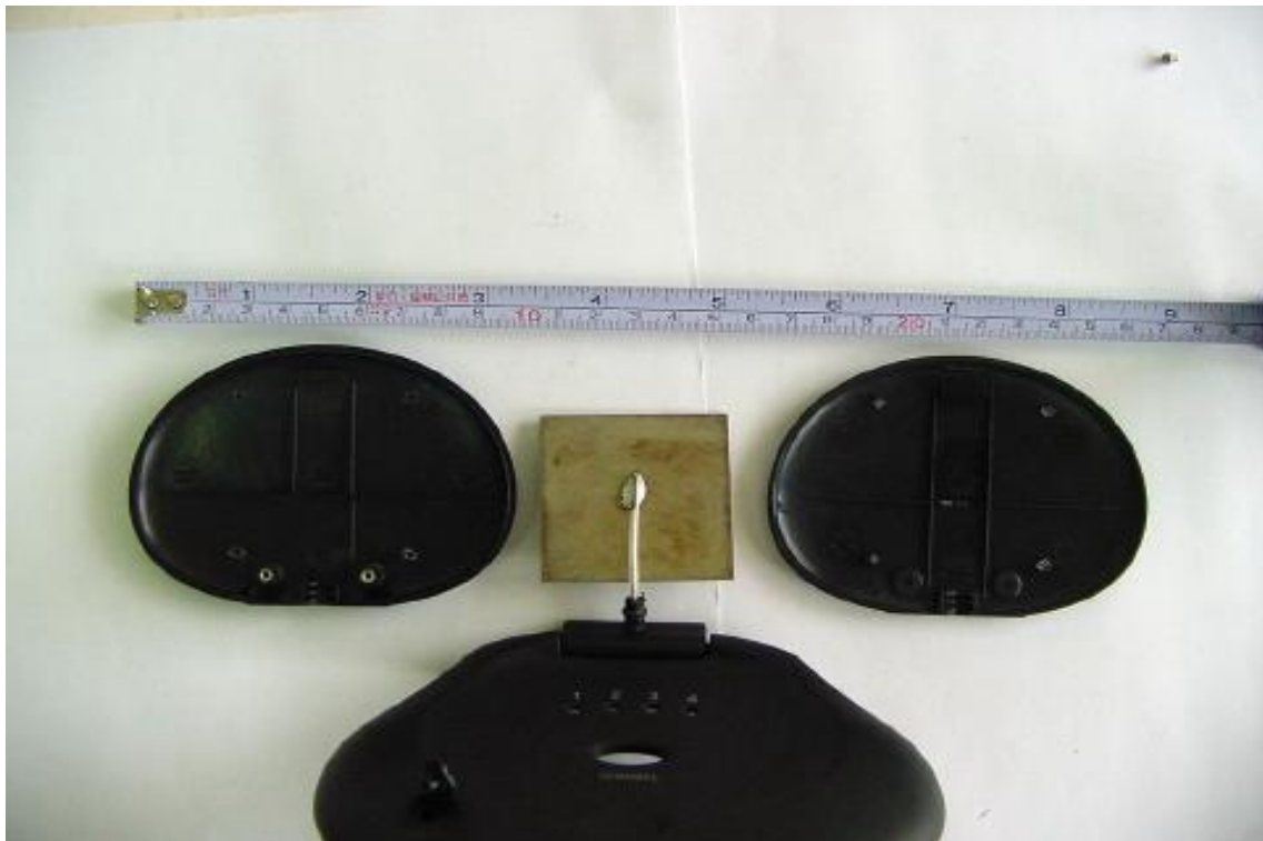
Internal View of Antenna
