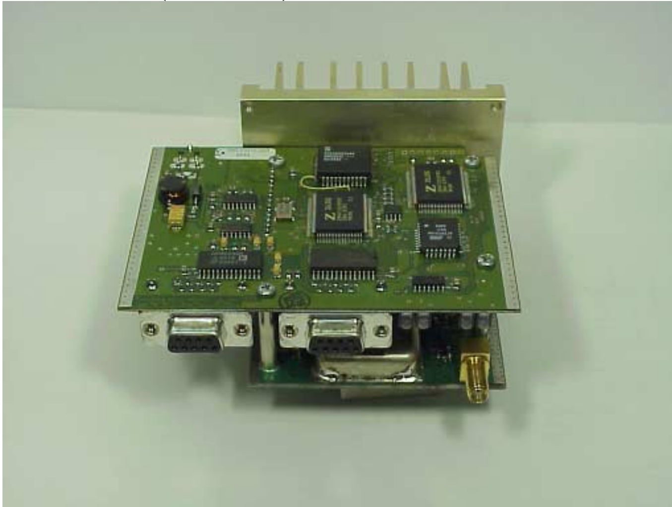
Photo 3: Internal (RF and Modem)
