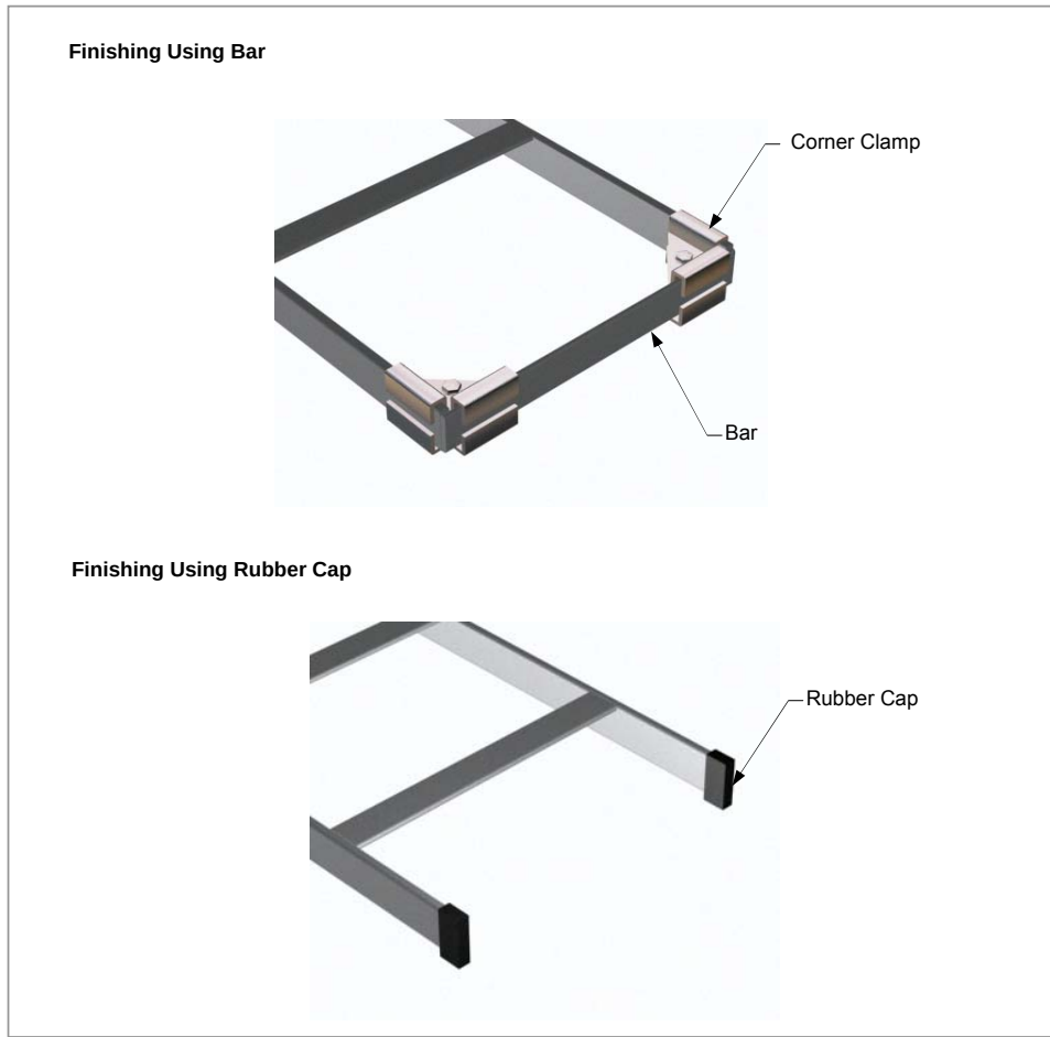
Figure 2.18 Cable Rack Finishing
