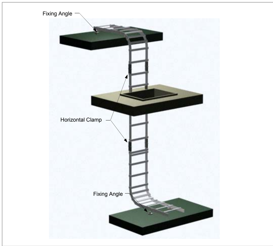
Figure 2.12 Installing Upper/Lower Curved Cable Rack
