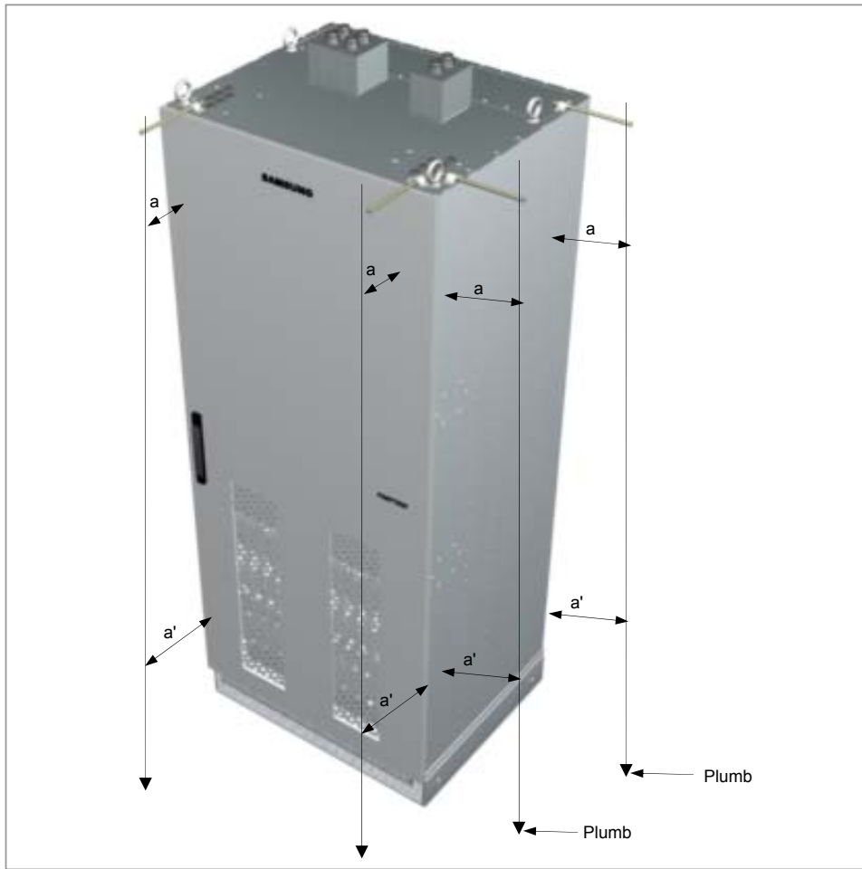
Figure 2.31 Leveling by a Plumb
