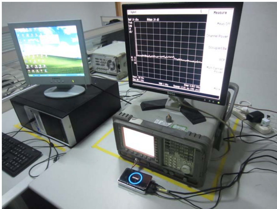
SPURIOUS EMISSION TEST SETUP
