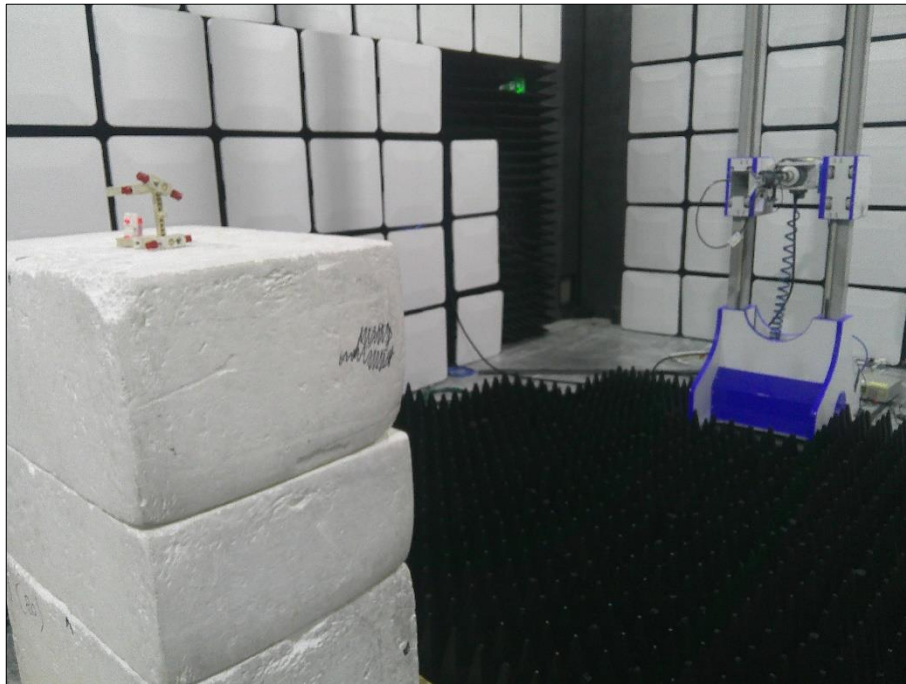
Figure 68 - Test Setup - 8 GHz to 18 GHz Z Plane
