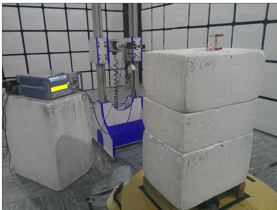
Figure 71 - Test Setup - 18 GHz to 25 GHz Z Plane
