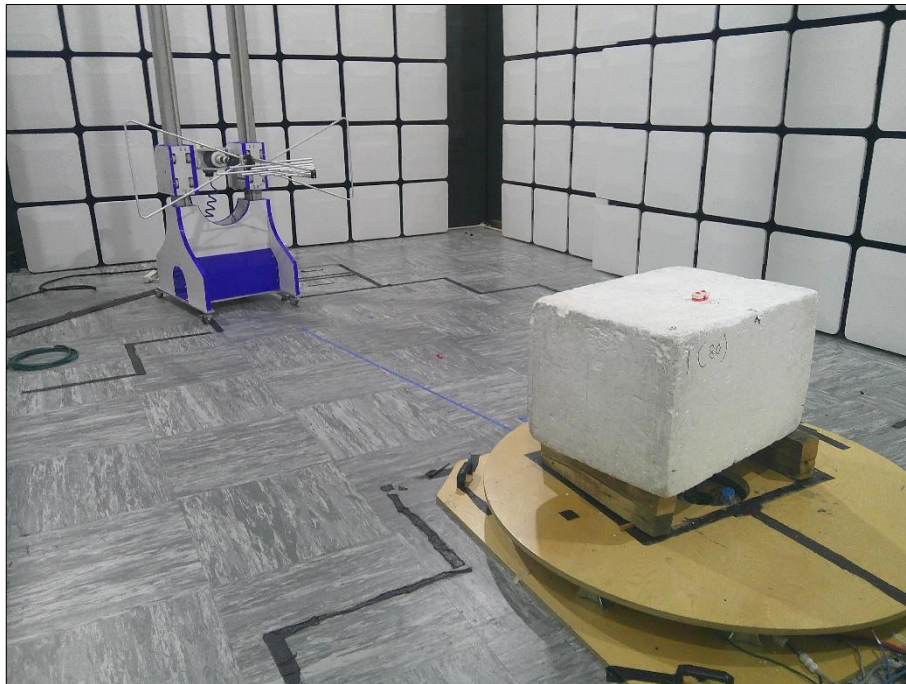
Figure 60 - Test Setup - 30 MHz to 1 GHz X Plane
