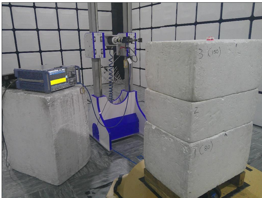
Figure 69 - Test Setup - 18 GHz to 25 GHz X Plane
