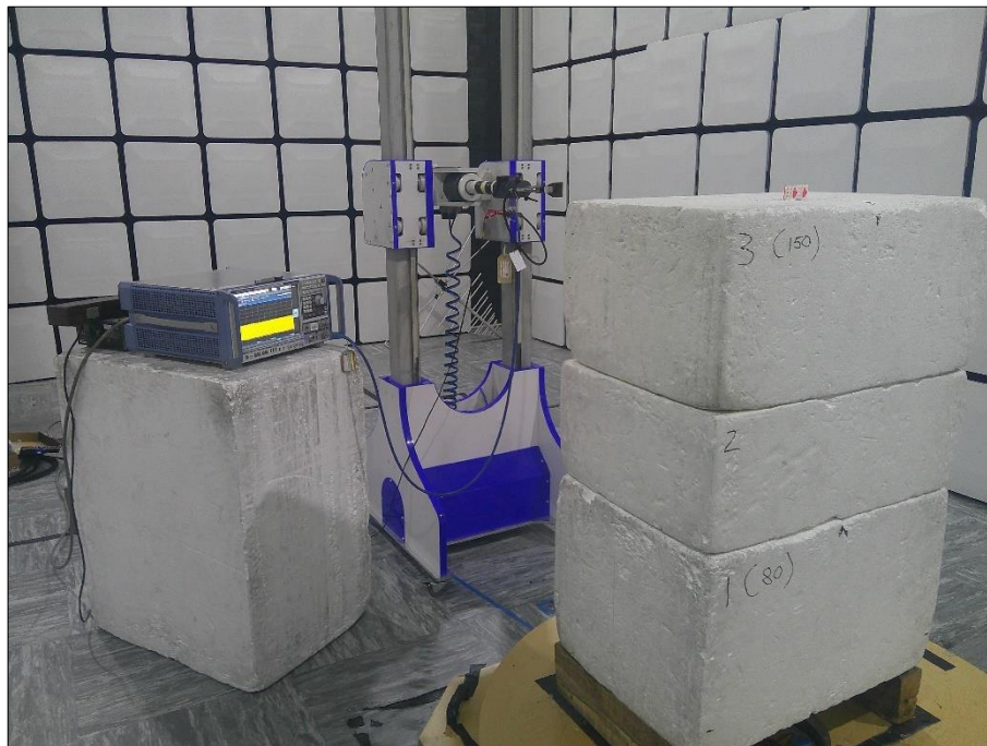
Figure 70 - Test Setup - 18 GHz to 25 GHz Y Plane
