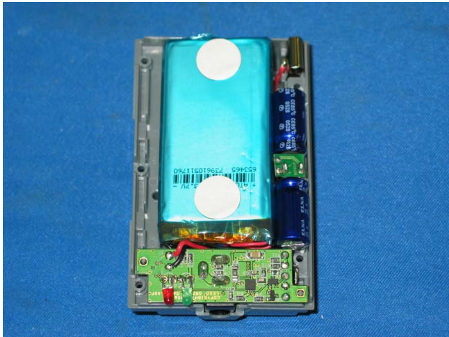
Rechargeable Battery Pack assembly
