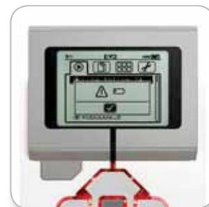
Low Battery Power Indicator
