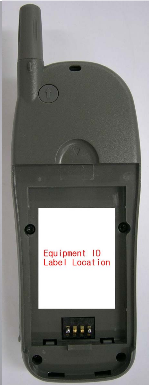
Rear View, with battery removed to show Equipment ID Label.
