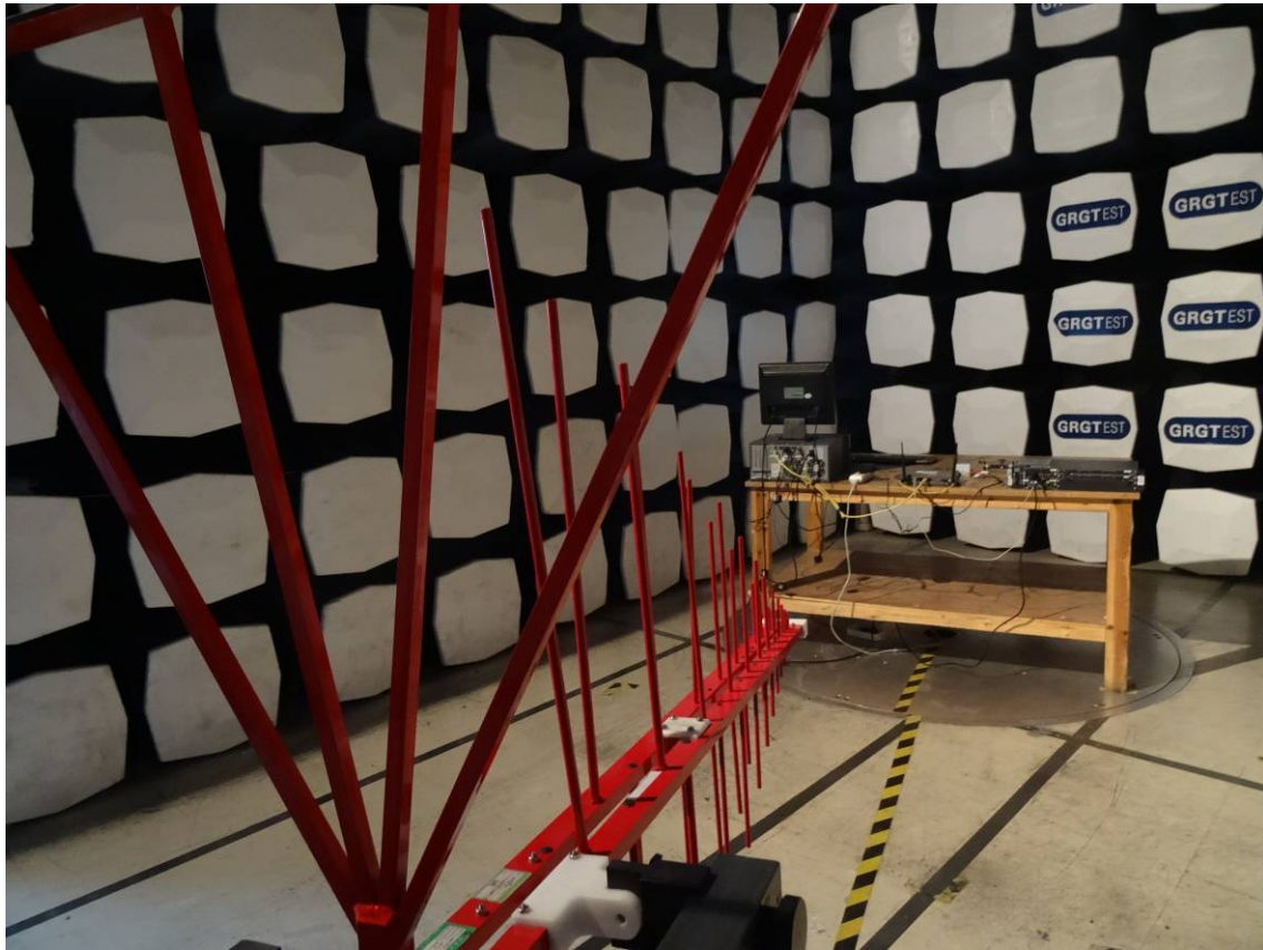
Radiated Emission (Below 1GHz)
