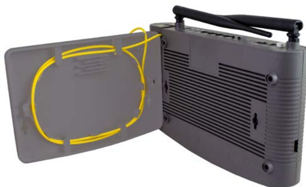
Figure 12 Snapping the ONT onto the Fiber Tray
