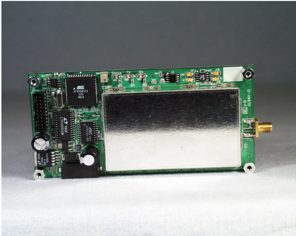
Front View of the Radio Board (with RF Can Installed)
