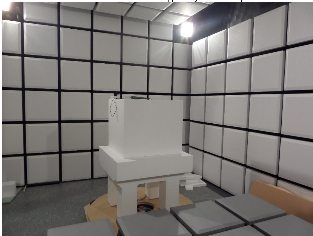
Anechoic room – Position 2 supplied by AC/DC Adapter
