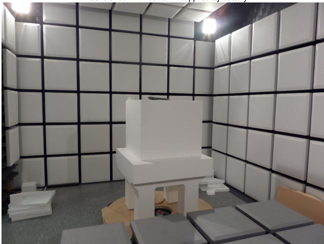
Anechoic room – Position 2 supplied by battery
