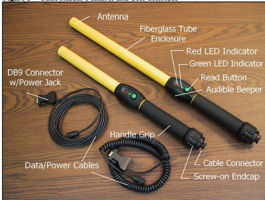
Figure 1 - Stick Reader Features and User Interface
