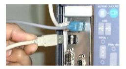
Connect the tablet's USB connector into an available USB port on your computer.
