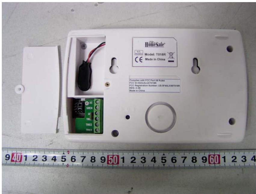
EUT – Battery Uncovered View
