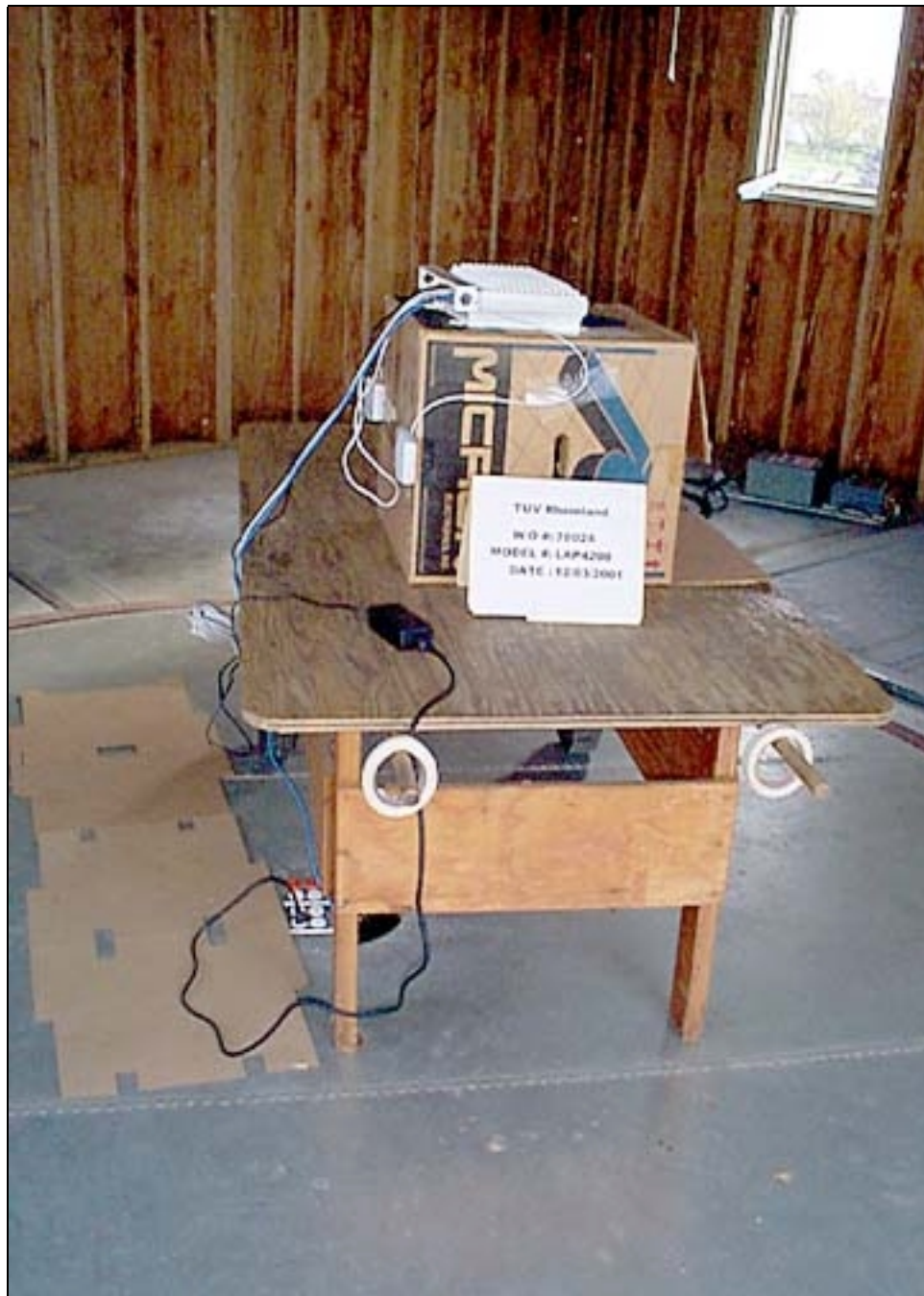
Radiated Emissions - Side View of LOS-4100 with AK-120 Antenna
