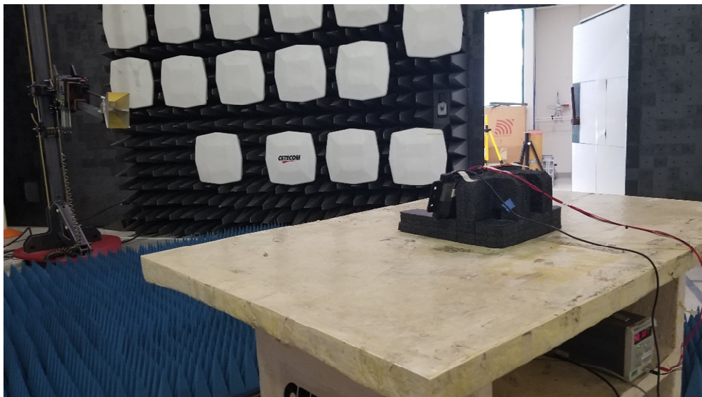
Photo 2: Emissions in frequency range 1-3 GHz
