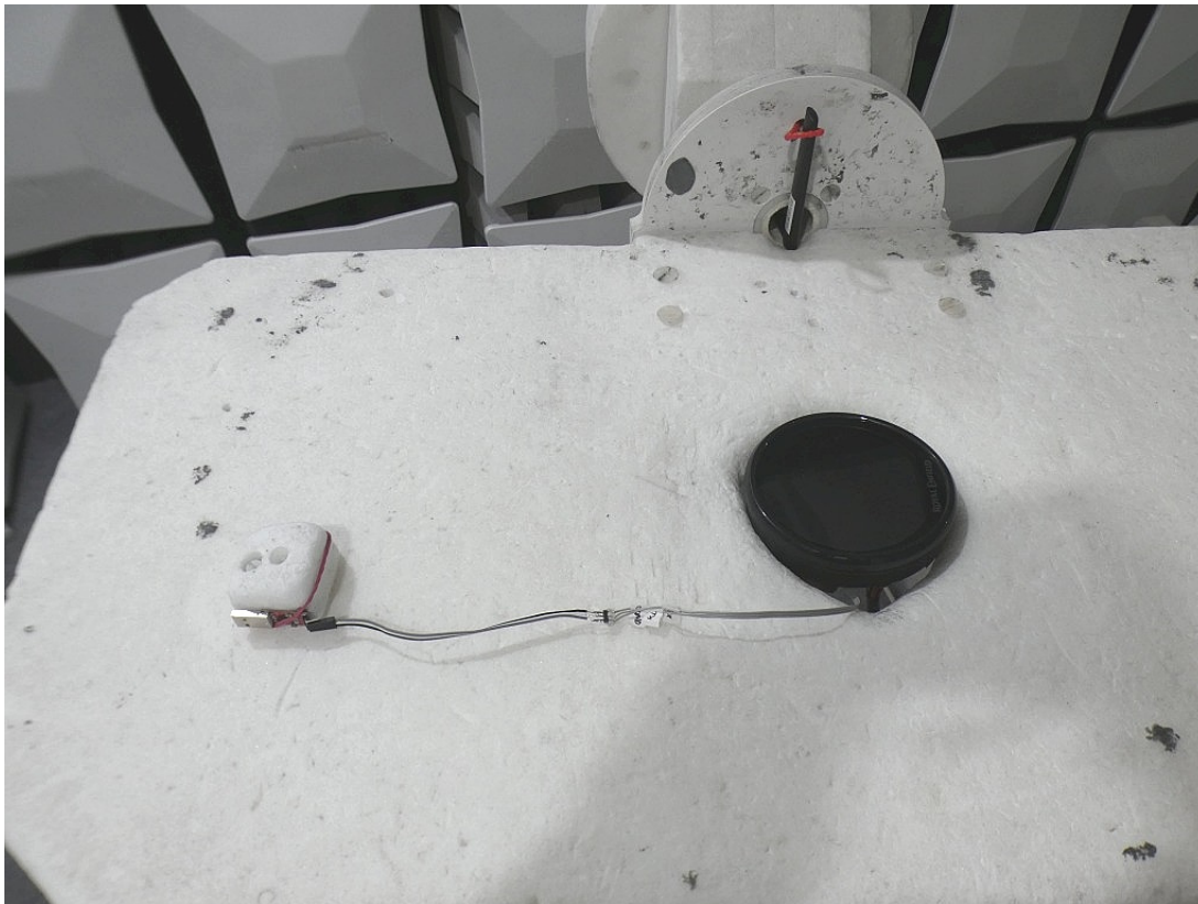
Photo 10: TTL-USB converter connected to EUT, but not supplied during tests
