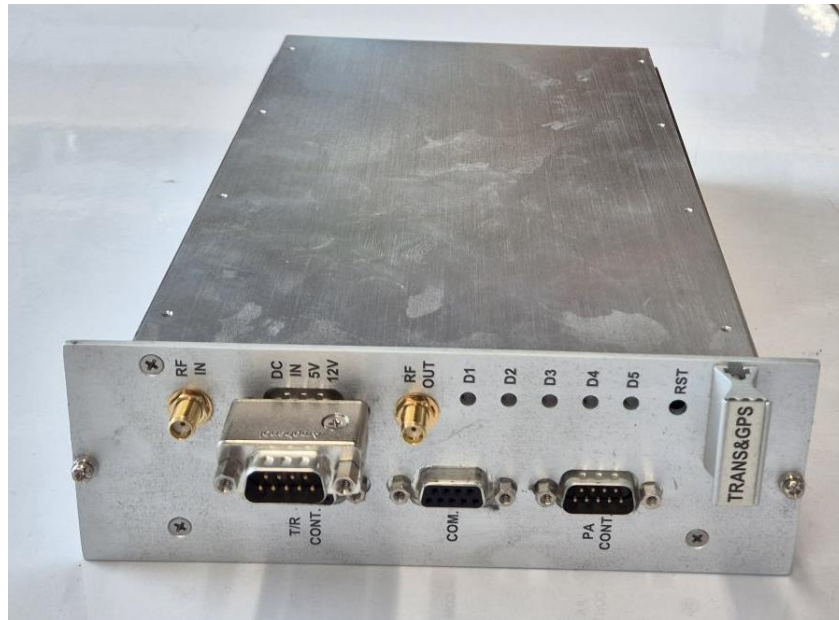
Galaxy Base Station V1- RF transceiver module
