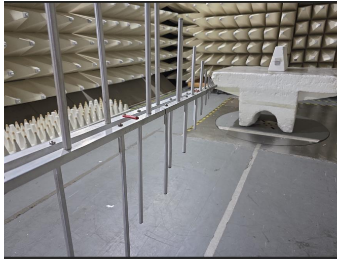
Photograph No.3 Setup for spurious emission measurements in the anechoic chamber above 30 MHz
