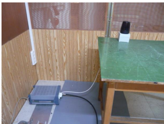
Photograph 7.9.1 Setup for conducted emission measurements
