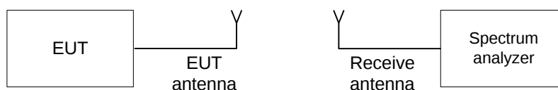
Figure 7.8.1 Band edge emission test setup
