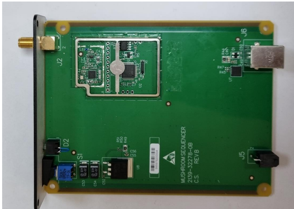
PCB Top without shield
